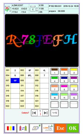
Press the number key to switch the ordinary head needle pole, Press Key switch to tape embroidery Head (limited function). The Embroidery box will automatically switch to the current head position.
